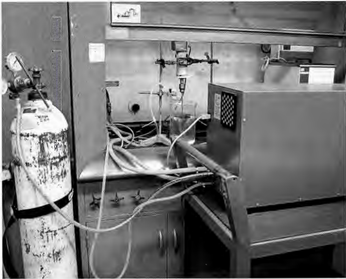
Figure 3.1. Laboratory set-up of ozonation.
